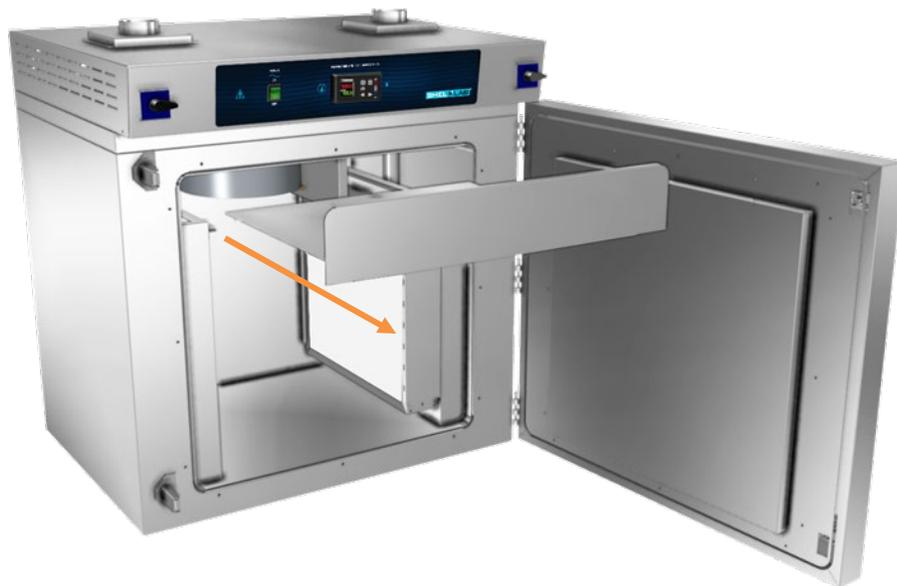
5. Remove the right wall air duct and filter.
