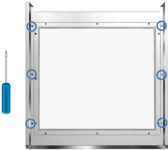
**6.** Loosen, but **do not remove**, the **6** screws on the air duct interior. This loosens the brackets that hold the filter in place.
