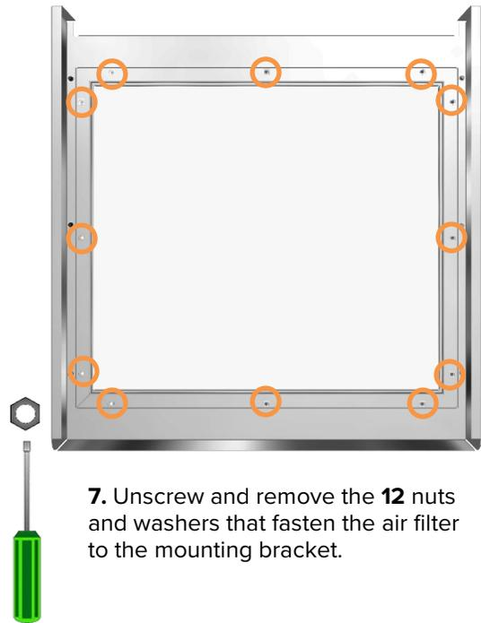
**7.** Unscrew and remove the **12** nuts and washers that fasten the air filter to the mounting bracket.
