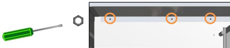
3. Unscrew and remove the nuts and washers located at the top of the back wall of the oven chamber.
