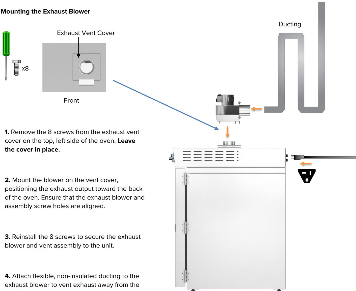
1. Remove the 8 screws from the exhaust vent cover on the top, left side of the oven. **Leave the cover in place.**
