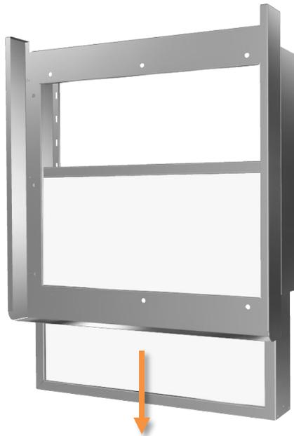
**8.** Slide the old air filter down and out of the air duct bracket.
