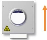
**3.** Secure the reference temperature device sensor probe at the center of the middle shelf, with the probe head 2 inches above the shelf surface.
