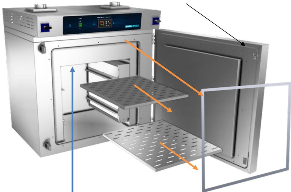
2. Remove the chamber gasket. It is difficult to remove the chamber liner components in the next steps without damaging the gasket if it is left in place.
